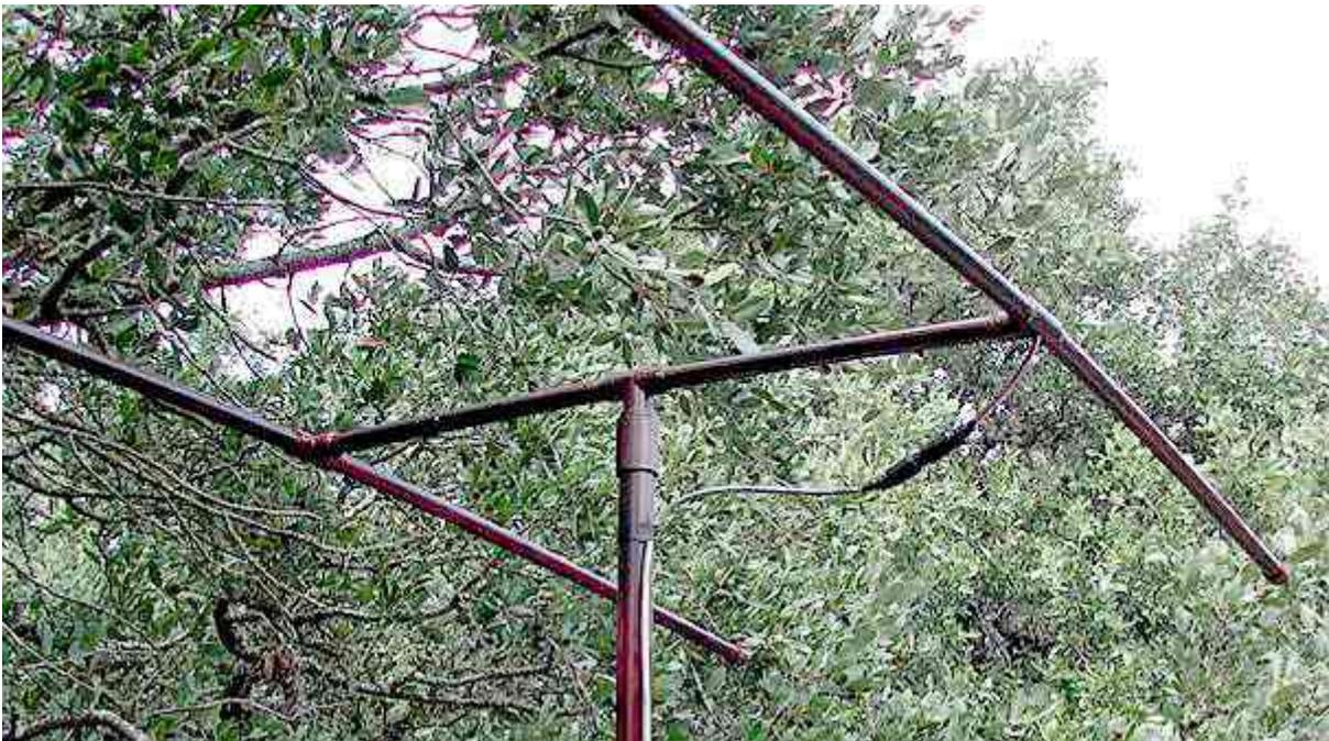
The 6 meter antenna has two elements and is housed in 1/2 inch pvc tubing, using T connectors to form the yagi configuration, and another T is located mid-way between the two elements for support. End caps are used to enclose the pvc ends. The coax feed is inserted into the DE T via a drilled hole on the T's under
