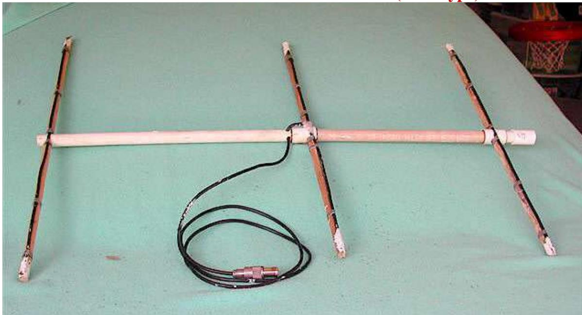
The 2 meter antenna in picture above is a three element yagi and again it uses John's formula for calculating the length for the DE and REF @ **146.0Mhz**.
