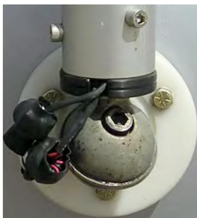
While controller and antenna manufacturers are very explicit about how these chokes should be installed, very few of them are installed correctly. Add in a little insult caused by improper mounting of the antenna in question (typically an inadequate image plane under the antenna), and RFI problems abound. Let's take a moment to look at ferrites.
