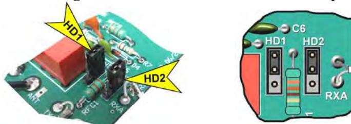
Figure 3 - Internal Jumpers HD1 and HD2
