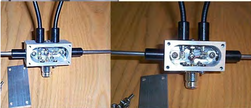
Ultra rugged box enclosure machined from a solid piece of aluminum rectangular stock. Walls are 1/8" thick, bottom 1/4".
