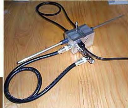
Polarity reversing unit measures 3 1/16" wide by 2 3/16" high by 2" wide.
