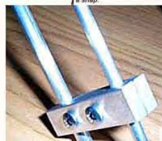
Two piece shorting bars held with machine screws and nylon insert nuts.
