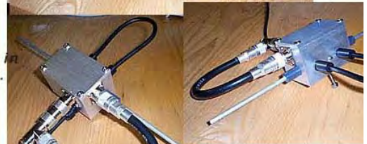
polarity reversing unit measures 2 3/16" high by 3 1/16" long by 2" wide
