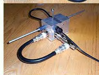
Element rods mount through black Delrin insulators. Assembly or disassembly is a snap.
