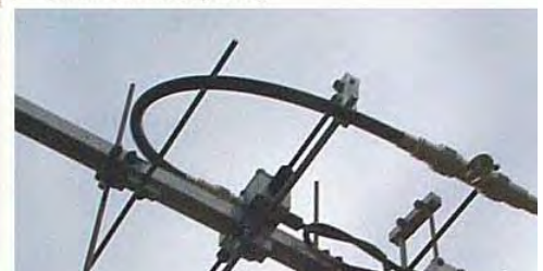
Two piece shorting bars held with machine screws and nylon insert nuts.
