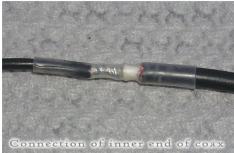
**Photo B** - Connection of inner end of coax section (closer to center).
