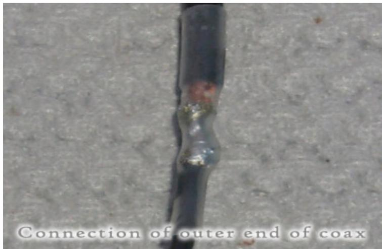
**Photo C** - Connection of outer end of coax section (further from center).
