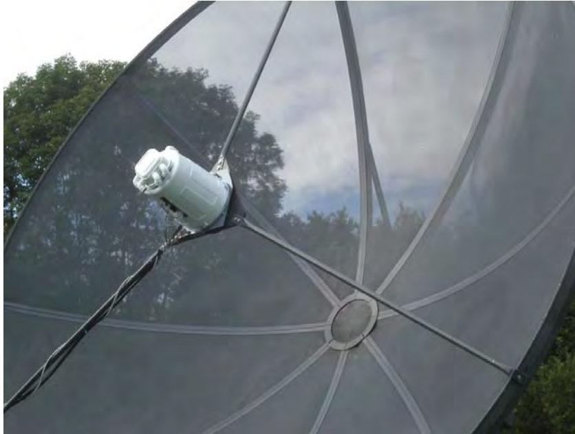
Figure 7 3m diameter dish with waveguide feed
