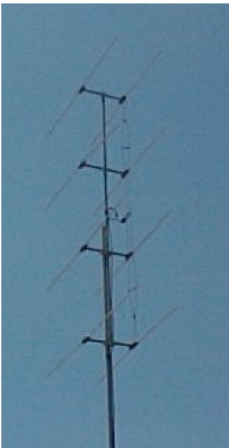
Figure 8. - four stacked half wave dipoles collinear antenna
