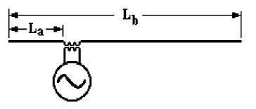
•The relationship between feed position and feed impedance is very complex, but in general as the feed moves towards away from the center, the impedance increases and the number of harmonics with low impedance resonance increases.
