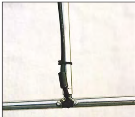
Figure 2 — Close-up of dipole electrical connections.
